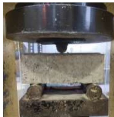
Figure 5: Flexural strength test setup
