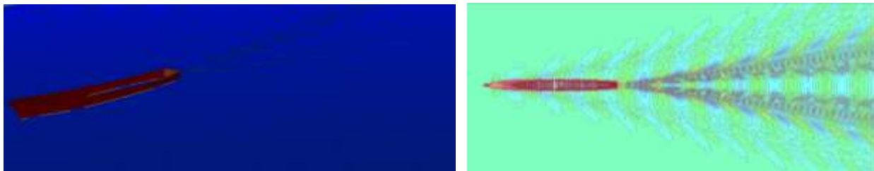
Figure 28 Free Surface Wave Contours for At Fn=0.40 - Medium Grid
