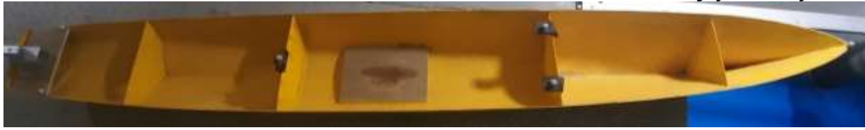
Figure 22 Model Subdivision—Dimensions Are in Ship Scale
