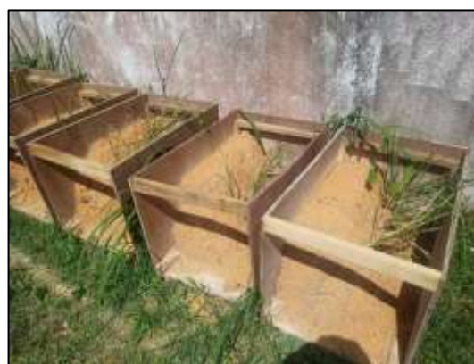
Figure 1: Physical Root- Soil Modelling with Varies of Slope Gradients
