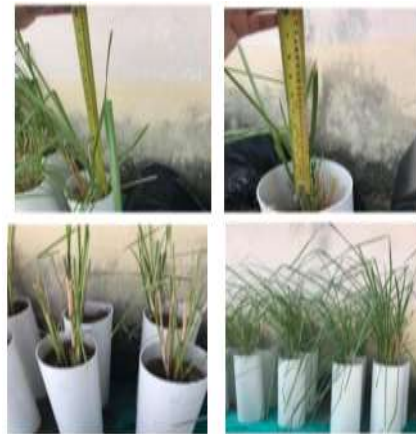
Figure 1: Vetiver grass was planted in PVC pipe – Physical Modeling
