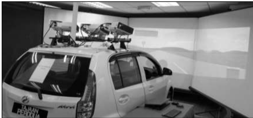
Figure 1: The consolidated CabinDS system
