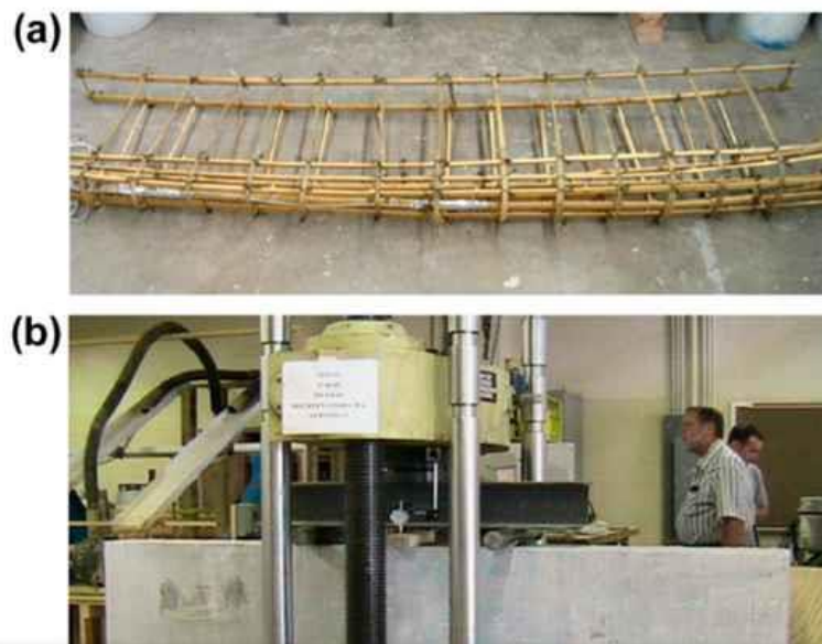
Figure 9. Concrete Beams Reinforced with Bamboo Rebars: (A) Finished Reinforcement, (B) The Setup [85]
